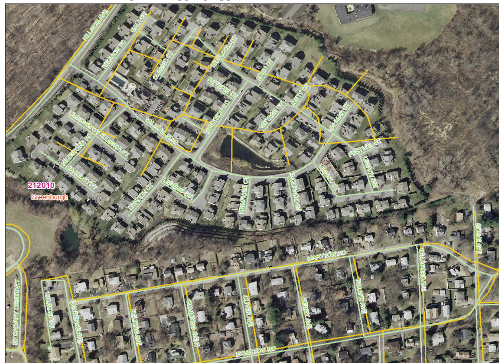
Data assembled with the original E911 street centerline file (orange) has been "conflated" to be more current and spatially accurate road centerlines (green).
