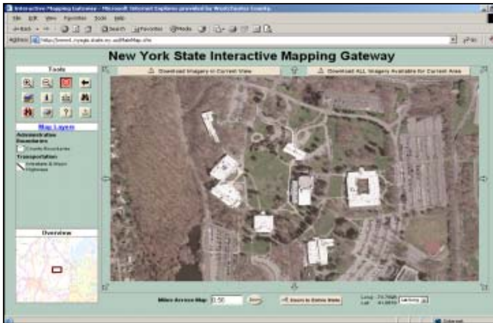
The state orthoimagery program provides data for download in both UTM Zone 18 and NAD 83 coordinate system and user options for downloading datasets are available depending on the type of user internet connection (modem vs. cable, etc).
