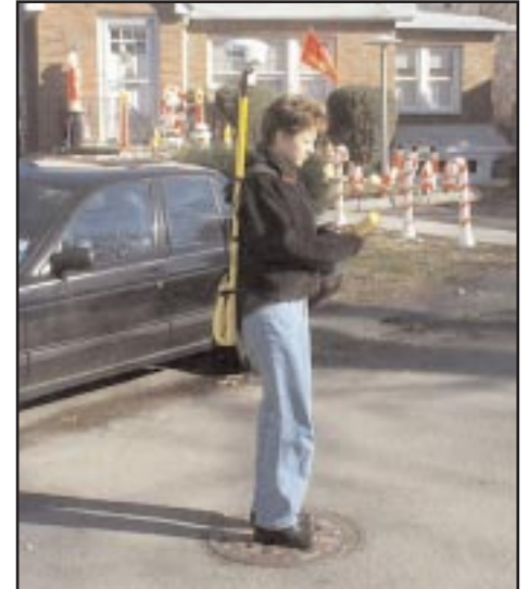
GIS staff, Laura McGinty, mapping a manhole location with a Trimble GPS unit on General Heath Avenue in North Castle.
